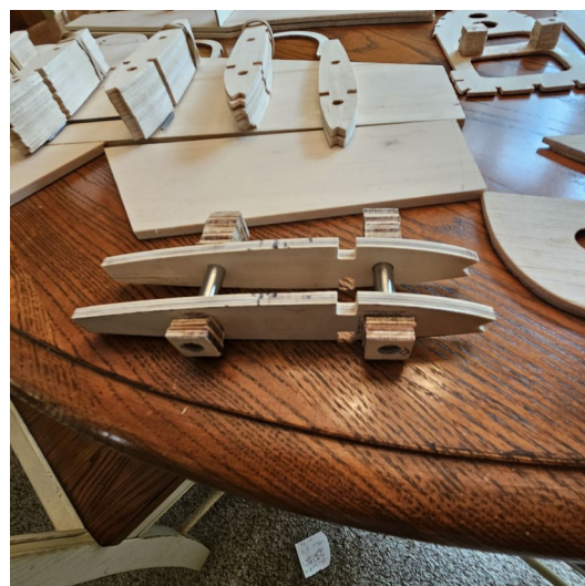
Wing rib jig for making several ribs at a time.
