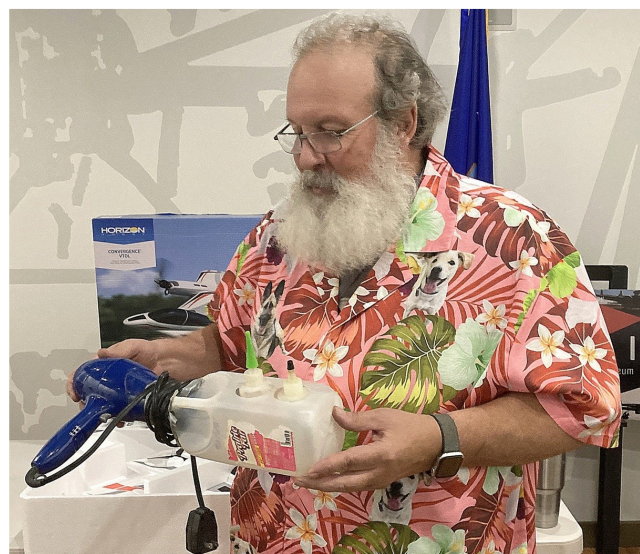
Mike Bealmear demonstrates how to heat and soften epoxy. The blue hair dryer directs hot air inside the modified milk bottle.
